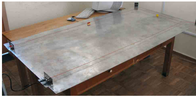
Fig. 1. Measurement setup for investigation of long (4.325 m) TWP cable
