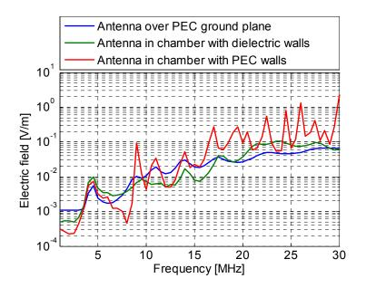
Fig. 5. Average electric field in reference points produced by log-periodic antenna
