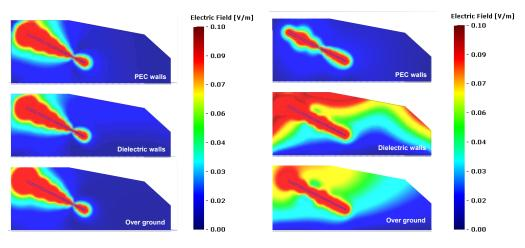
Fig. 7. Electric field at frequency 5 MHz
