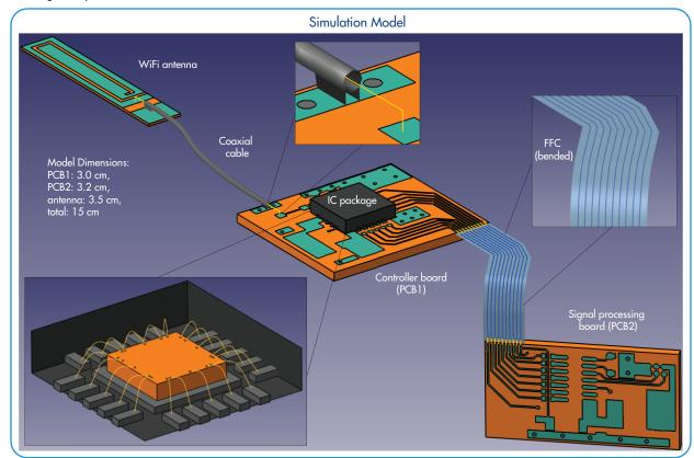
Physical properties of the model are shown below. FR-4, FR-35 and silicon dielectric materials are used for PCBs, antenna and IC package substrates correspondingly. The copper is used as a conductor material.
